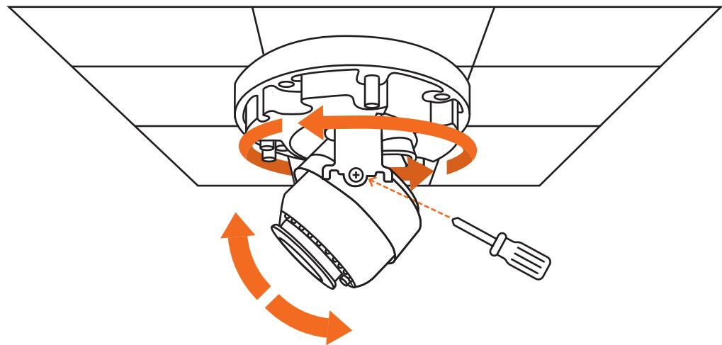
6. Rotate the camera when the images are at an angle or upside down.
