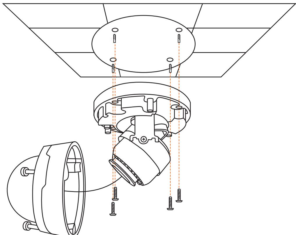
5. Turn the camera left or right. Loosen the screws at the side to move the camera up or down.
