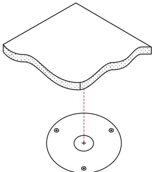
4. Place the bracket and fasten it with screws.
