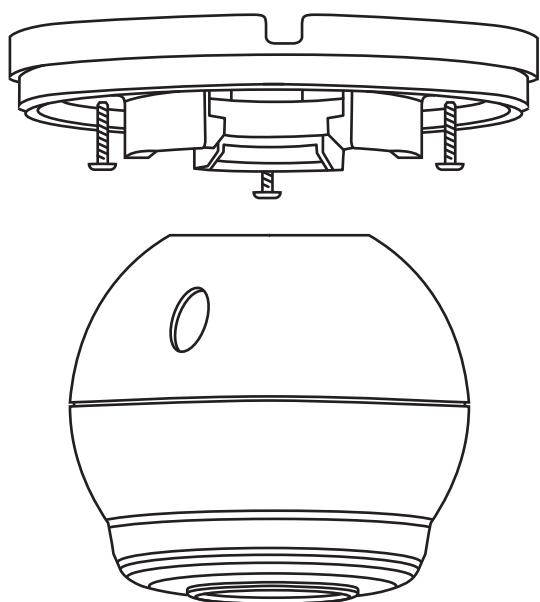
5. Bring the camera in the right position and install the bracket.
