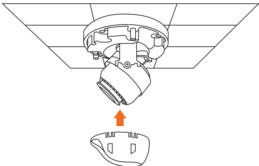
9. Replace the front cover and tighten the screws.
