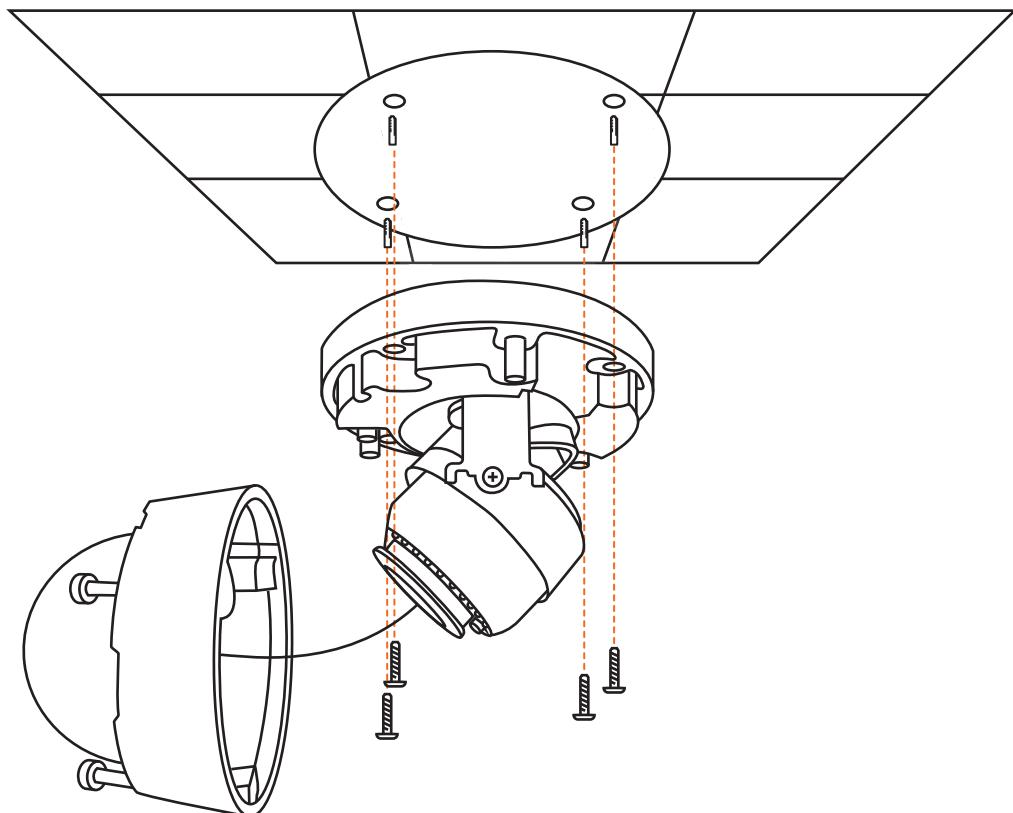
5. Turn the camera left or right. Loosen the screws at the side to move the camera up or down.
