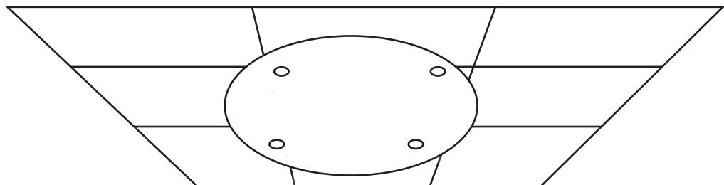
4. Drill the holes and mount the camera. Use expansion bolts and locking screws.
